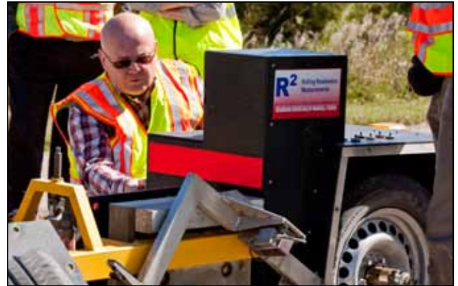
Professor Jerzy Ejsmont from Gdansk, Poland, prepares equipment to measure pavement rolling resistance at MnROAD.
