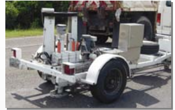
Falling Weight Deflectometer - FWD
